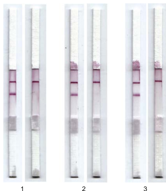
Fig. 6. Immunochromatographic detection of ofloxacin in milk with a fat content of 3.5% (1), chicken meat (2), and pork (3). The left test strip for each matrix corresponds to the absence of ofloxacin, and the right strip corresponds to the presence of ofloxacin at a concentration of 30 ng mL -1 .
